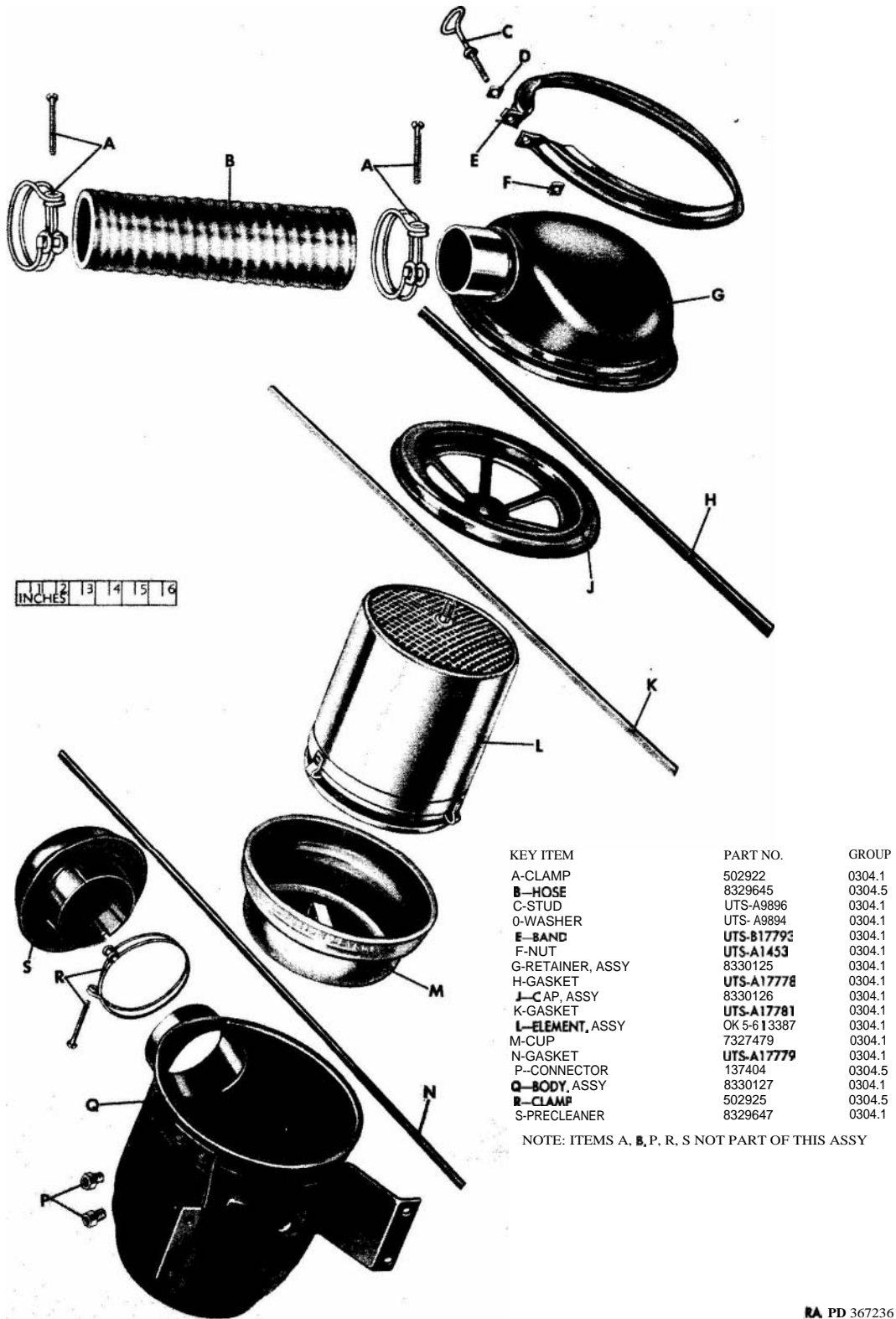
Figure 03-6. Air cleaner, assy (8329642)—exploded view
