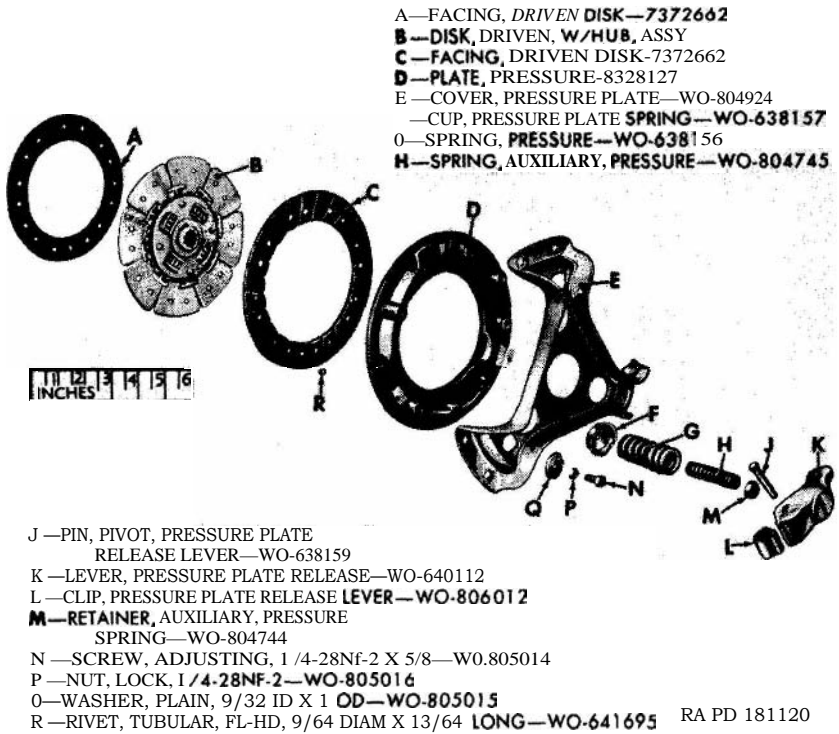
Figure 109. Clutch, assembly-disassembled view.
