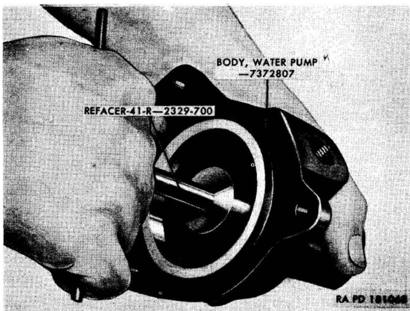
Figure 57. Refacing water pump body teal surface using refacer 41-R-2329-700.
