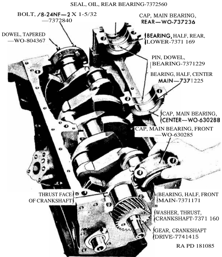
Figure 74. Installing main bearing halves in main bearing caps.
