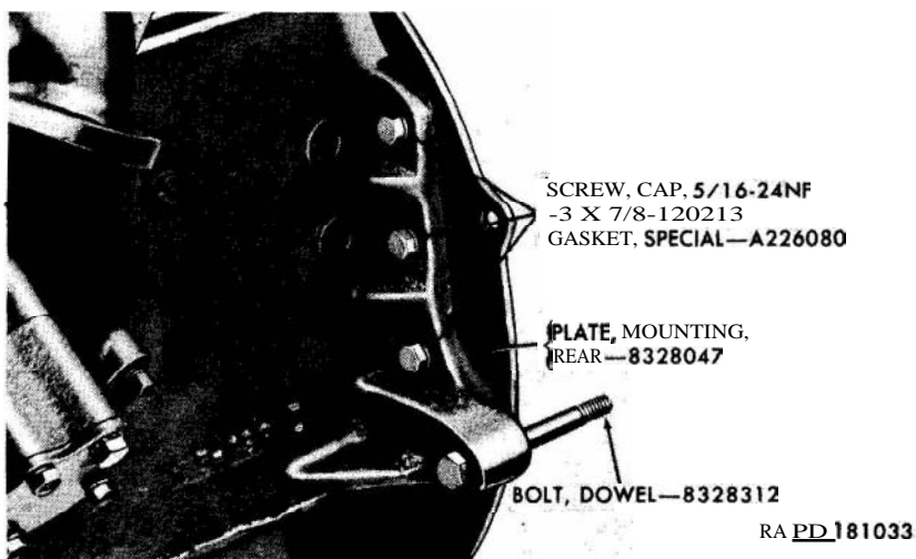
Figure 22. Location of rear mounting plate cap screws—left side of engine.
