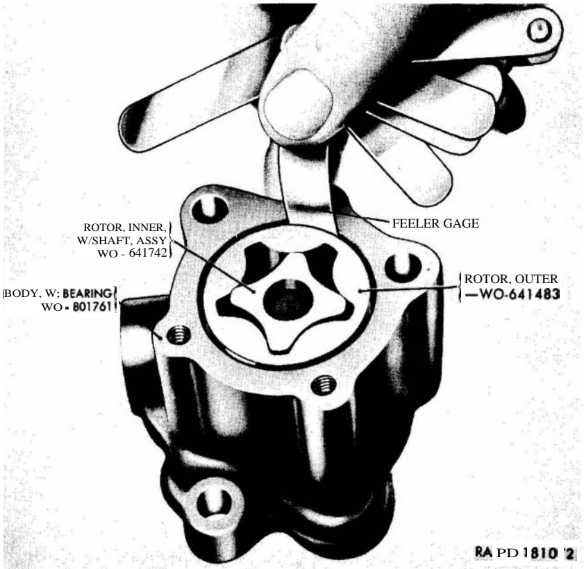
Figuer 61. Checking outer rotor to oil pump body clearance.
